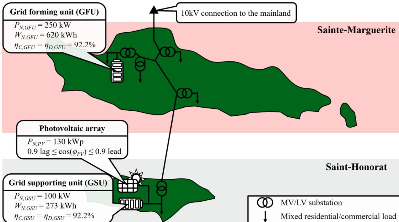
Fig. 1 Depiction of the Lérins' Islands, the MV grid section and the relevant DER.
