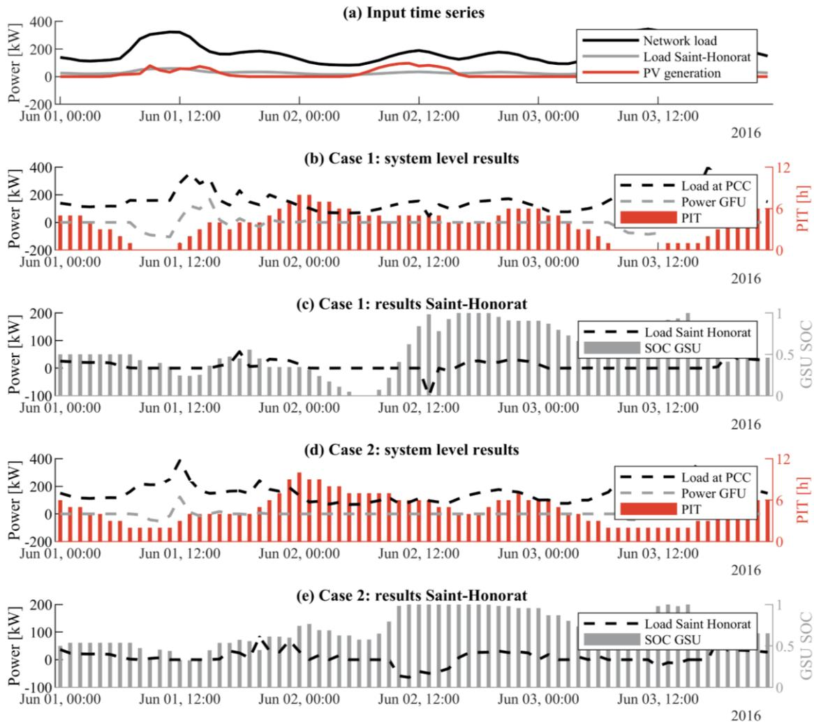
Fig. 1 Input data and simulation results: (a) 72 h input time series of network load, PV generation and load at Saint-Honorat; (b) Time series of optimized load at the PCC and GSU, as well as PIT in case 1; (c) Optimized load time series of load at Saint-Honorat and SOC of GSU in case 1; (d) Time series of optimized load at the PCC and GSU, as well as PIT in case 2; (e) Optimized load time series of load at Saint-Honorat and SOC of GSU in case 2
